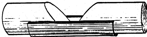
Butt weld in flat position
